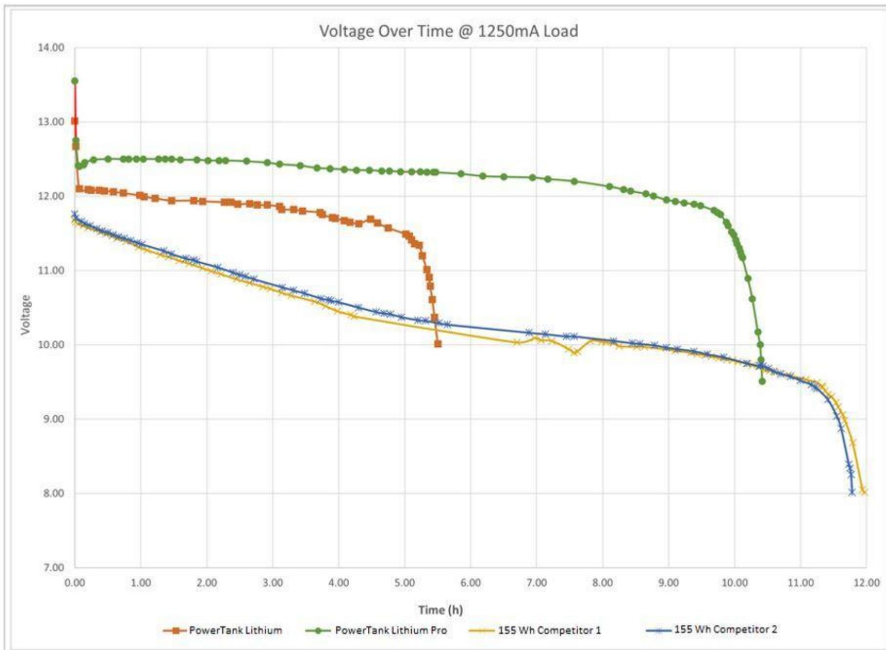
Celestron tested voltage over time for PowerTank Lithium, PowerTank Lithium Pro, and two competitors' batteries.
